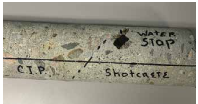
Fig. 2: Core sample from a pool that had the floor cast-in-place and the walls shotcreted
