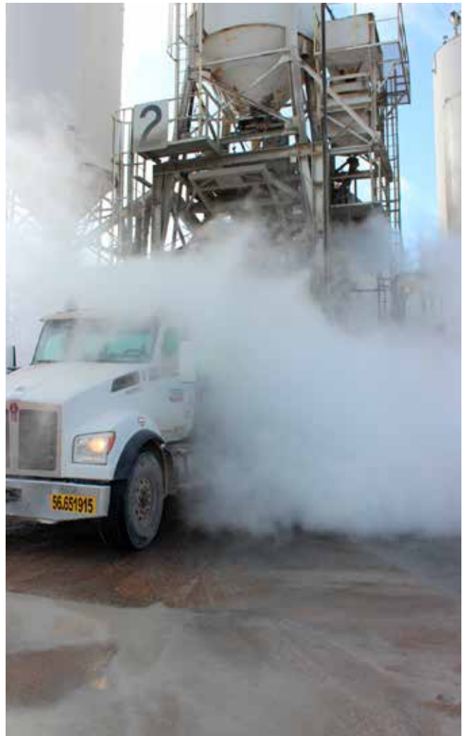
Fig. 4: As liquid nitrogen hits the warm aggregate, it instantly becomes a harmless nitrogen gas
