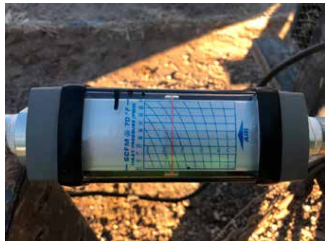
Figs. 1 and 2: Manometer (ABOVE) for pressure measure and flowmeter (BELOW) for airflow measurement
