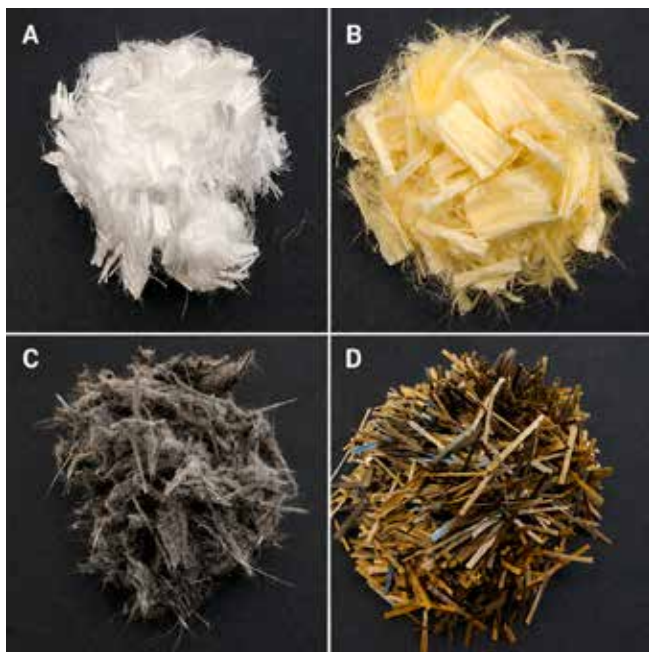
Fig. 3: An example of different microfiber chemistry: A) Polypropylene; B) Acrylic; C) Recycled Carbon Fiber; D) Basalt
