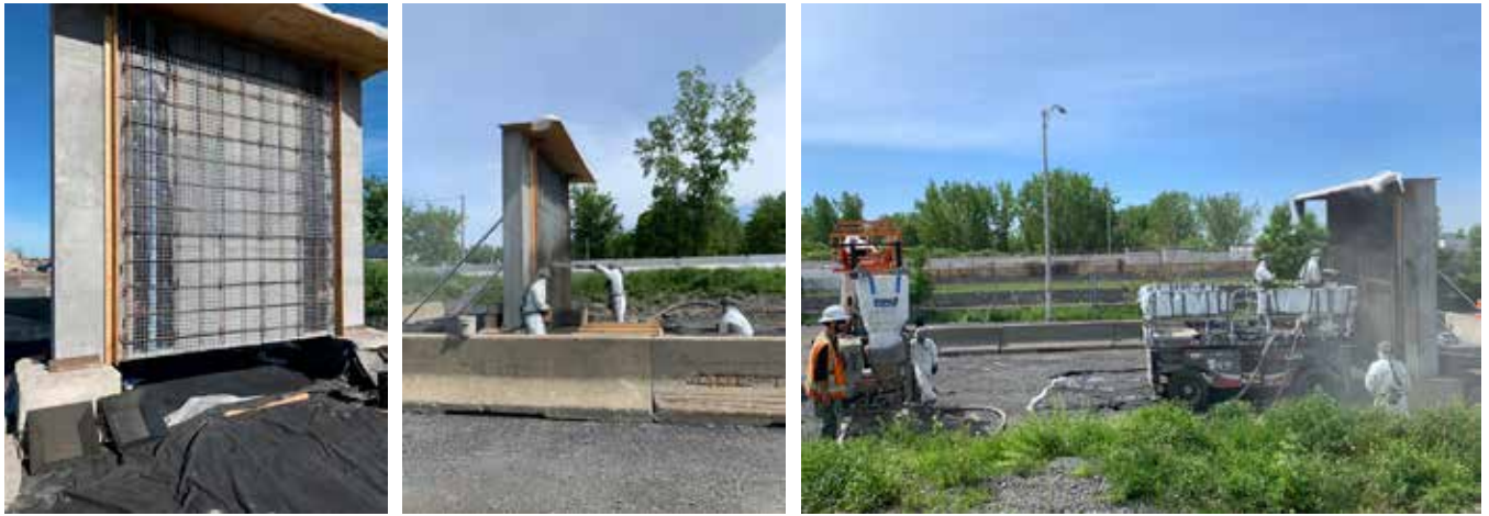
Fig. 7: Preparation of the panel with dry-mix shotcrete King® MS-D1 FSR for the HCM fire curve testing by the contractor Groupe LB. Photo credit: Sika Canada (2022).
