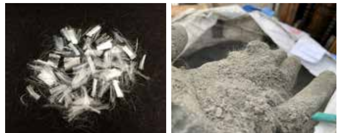
Fig. 6: Close-up views of the fibers in Sika® Fibermesh® 150F, a fiber designed to prevent explosive fire spalling in concrete. Photo credit: Sika Canada (2023).
