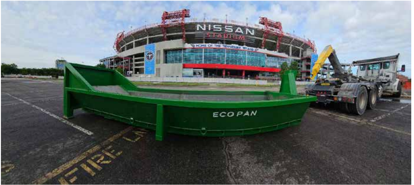
10 yd 3 (7.6 m 3 ) roll off at Nissan Stadium project in TN
