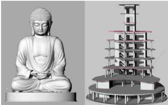
Fig. 1: Concept design of statue and interior support
