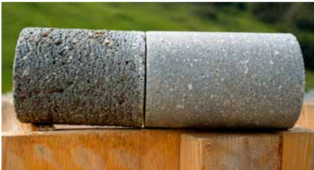
Fig. 1: Two cores (by two different shotcreters with the same concrete mixture) produce two very different results
