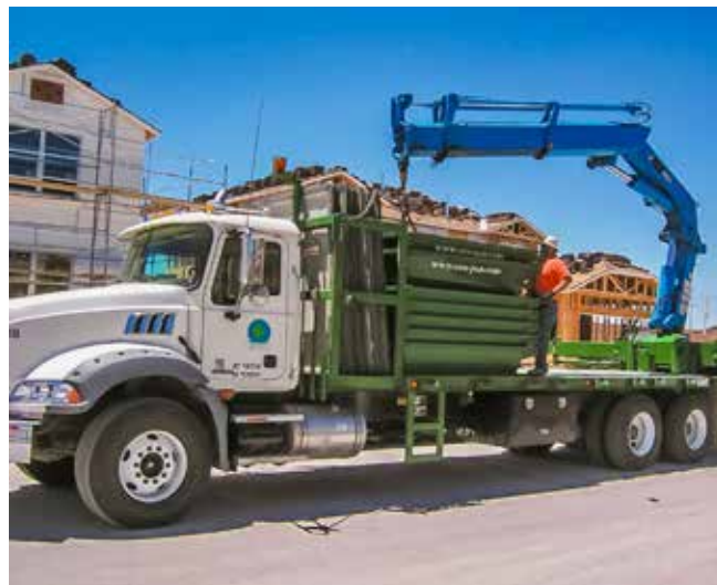
ECO-PAN crane truck unloading pump pans at a residential site
