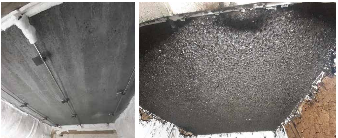
Fig. 8: HCM testing panel before (LEFT) and after (RIGHT) being exposed to 2372°F (1300°C) for 180 minutes. No visible damage was reported after testing. Photo credit: CERIB (2023).
