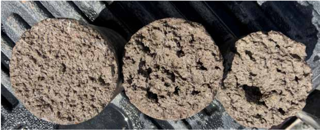
Fig. 7: Distance results from left to right — good distance, too far, and too close
