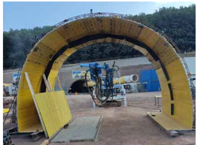
Fig. 2: Test setups of the artificial tunnel profiles for the initial tests
