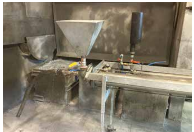
LabSprayer: Two funnels are visible. The grey funnel connects to the larger cylinder for mortar, and the black funnel connects to the smaller cylinder for admixtures. The mixing between the mortar and the air-accelerator blend takes place in the nozzle at the end of the hose, visible in the picture.
