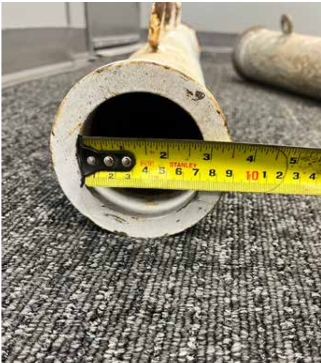
Figs. 6 & 7: When comparing the new and used pipes side by side, there's a noticeable difference in diameter. Upon measuring, it's clear that the used pipe is slightly larger.
