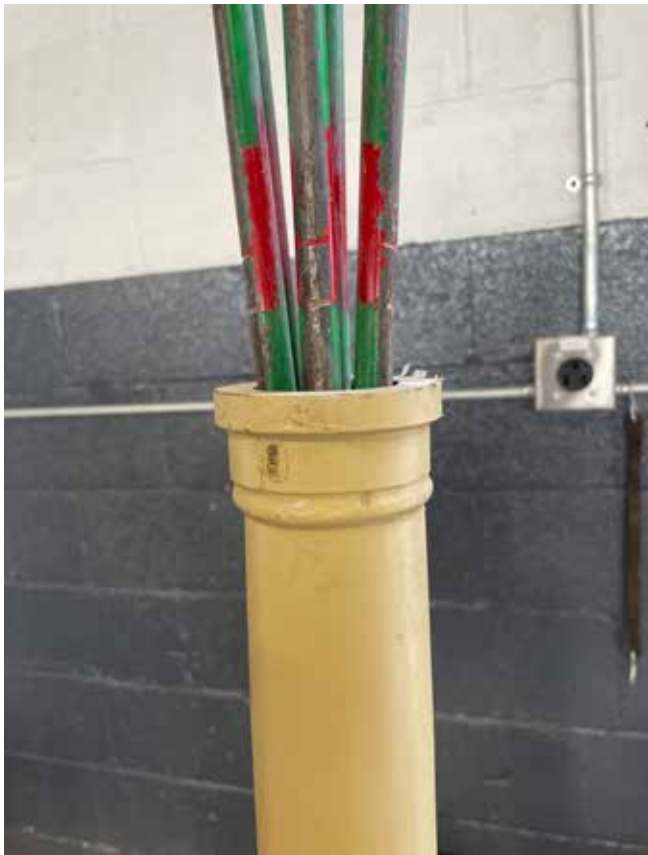
Figs. 9 & 10: Here we can see that the pipe that has been in service is now at the red marking, indicating no longer safe for use.
