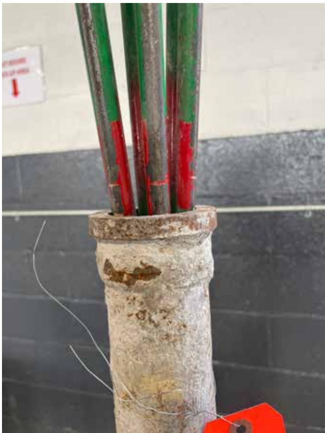
Figs. 9 & 10: Here we can see that the pipe that has been in service is now at the red marking, indicating no longer safe for use.
