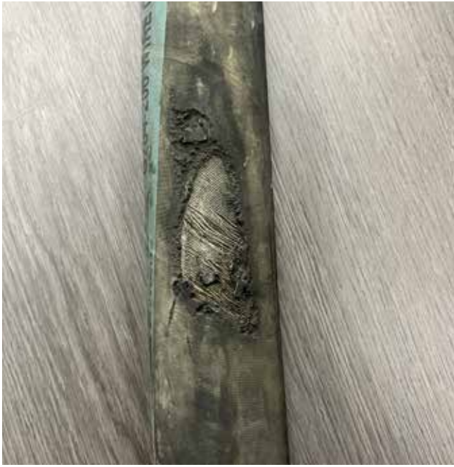
Fig. 3: 'Down line' hoses, which are connected to the reducer at the pump, are wire-braided to handle higher pressure. This particular hose shows a clearly worn area, likely caused by repeated contact with a soldier pile.
