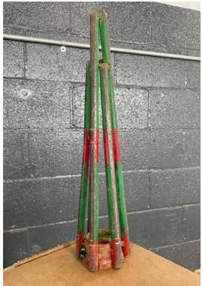
Fig. 8: Consolidated Shotcrete designed an inspection tool to evaluate pipe condition and determine end-of-life criteria.”
