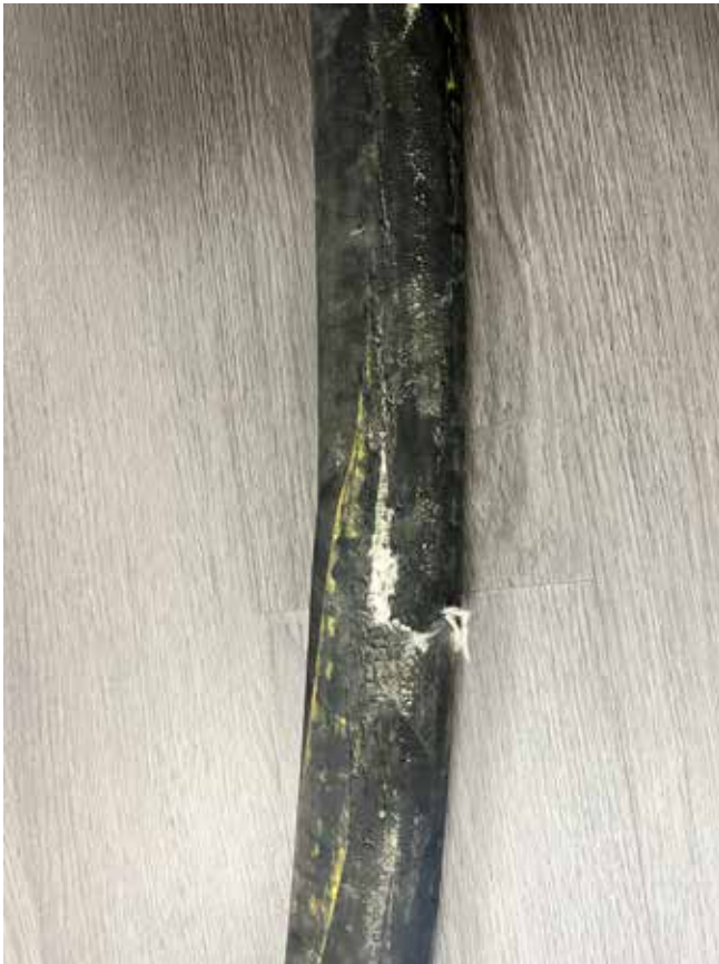
Fig. 4: This material line suffered a rupture; upon inspection it's noticed that this section was showing clear indentations. These were likely caused by repeated rubbing against rebar. This caused a weakened section in the line and ruptured during a plug.
