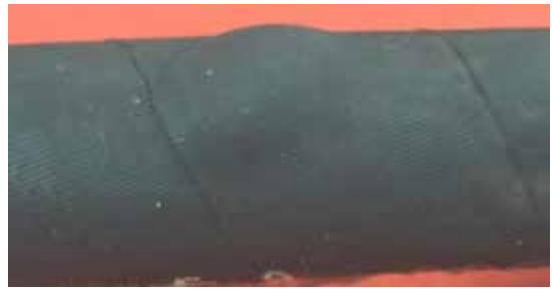
Fig. 3: Bulge in outer hose jacket exposing a 'soft spot' in the hose
