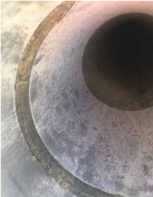
Fig. 2: Hose body worn through, exposing the hose beneath it; can be seen and felt as a bumpy wear pattern by using your fingers
