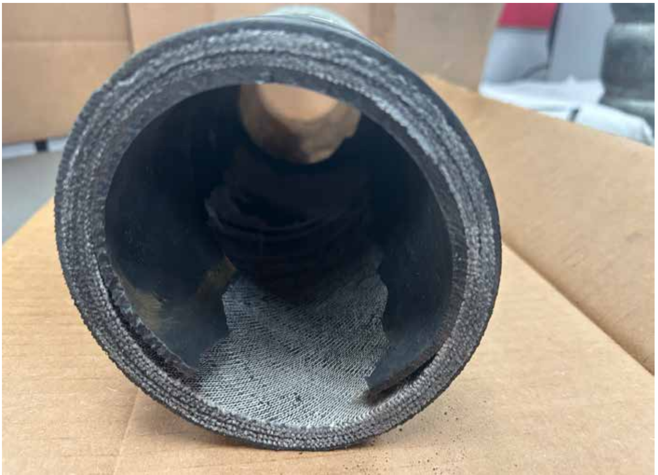
Fig. 1: Fabric reinforcement exposed, inner wear liner missing
