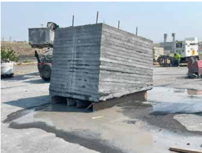
Mock-up block stripped and lowered to the ground for evaluation
