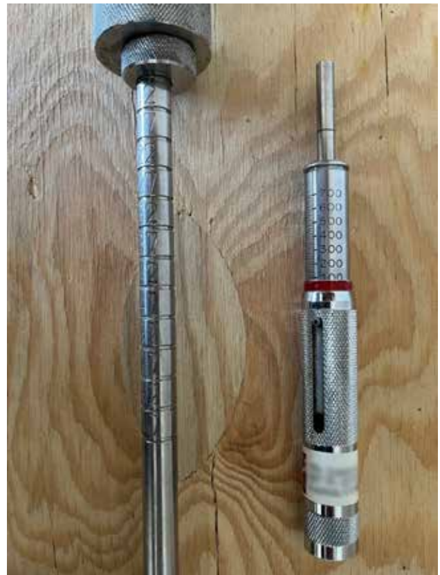
ABOVE: Soil penetrometer top (smaller) Needle penetrometer bottom (larger)
