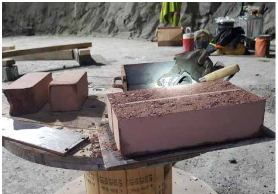
End beam sample removed from form ready for testing
