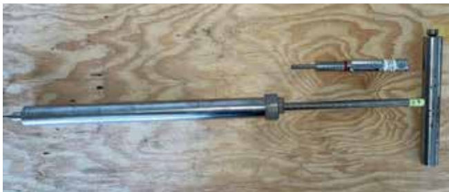
ABOVE: Soil penetrometer top (smaller) Needle penetrometer bottom (larger)
