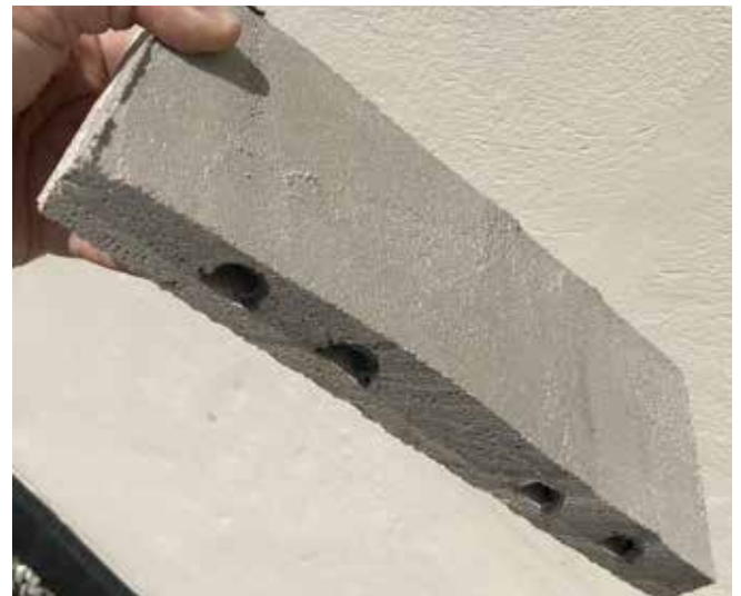
Fig. 4b: Application of Dolenco Drain: Cross section of shotcreted sample showing a network of channels that lead water away, alleviating pressure.
