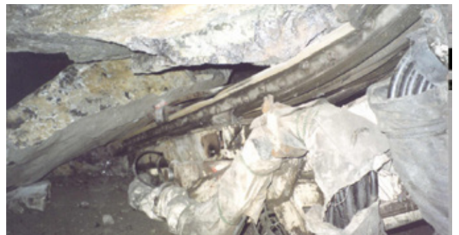
Fig. 1. Rock fall on jumbo equipment
