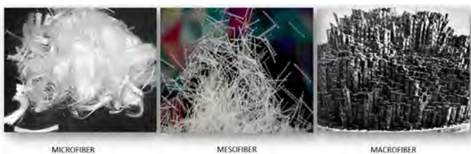
Fig 3: Typical synthetic microfibers, mesofibers and macrofibers
