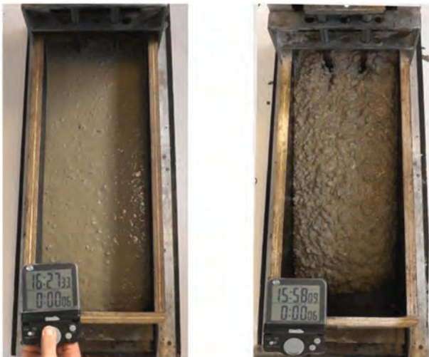
Fig. 1: MASTEREASE VS. PCE SUPERPLASTICIZER - L-box flowability test results show the improved placement characteristics of a MasterEase (left, six-second flow) mix versus one dosed with a polycarboxylate ether superplasticizer (right, 22-second flow). Both specimens bear the same mix designs and target slumps.
