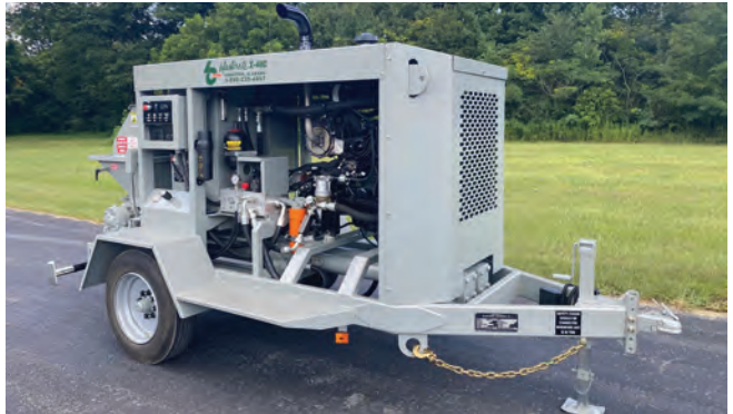
Fig. 3: The X-40D pump boasts 1,000 psi of piston face pressure, with a 5-inch discharge and the ability to put out 40 cubic yards of concrete per hour. Blastcrete engineered it for minimal maintenance to limit downtime.
