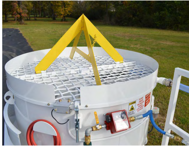
Fig. 4: Bag slicer for 2,200 bulk bags of pre-packaged refractory
