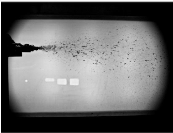
Fig. 3a: LVSM particles spray at 5 CFM with nozzle no. 1—recorded image for speed calculation.
