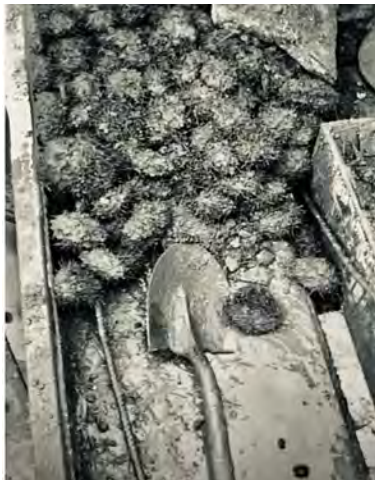
Fig 12: Balling up of fibers introduced into a concrete mixture
