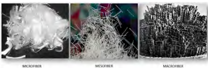
Fig 3: Typical synthetic microfibers, mesofibers and macrofibers
