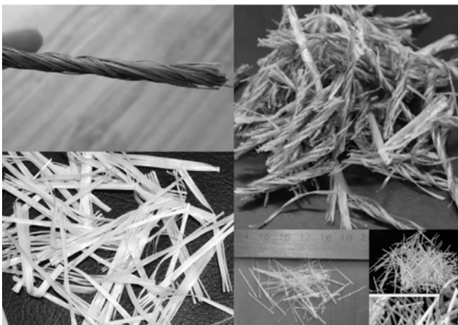
Fig 8: Smooth synthetic fibers with a rectangular shape
