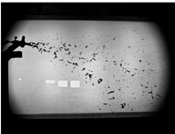
Fig. 4a: LVSM particles spray at 11 CFM with nozzle no. 2—recorded image for speed calculation.
