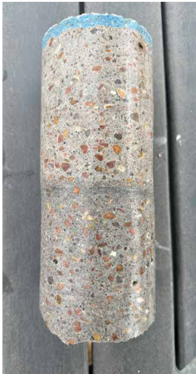
Fig. 1: Core sample taken through the floor of a pool near the cove showing unconsolidated layering.
