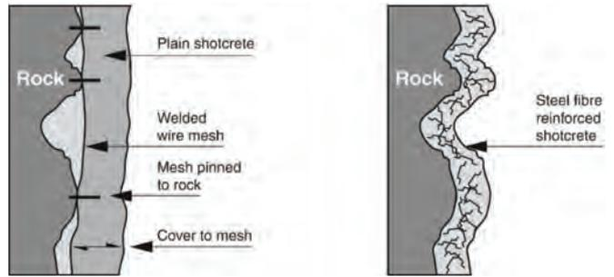
Figure 1: Rebar vs. SFRC Reinforcement.
