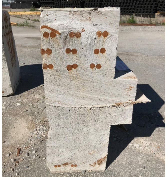
Fig. 8: A wire saw cut section of mockup showing excellent consolidation of shotcrete around the three layers of #35M (#11) rebar at the back of the work and to the outer membrane next to the embedded plastic water stop. Credit: Jimmy Wang.
