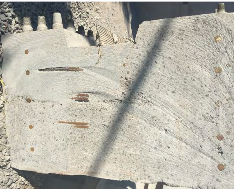
Fig. 23: An example of a wire saw cut section of mockup showing excellent quality of shotcrete at the transition between the shotcrete and the SCC using the StayForm Option 1 at the roof soffit with the keyway and plastic embedded water stop detail
