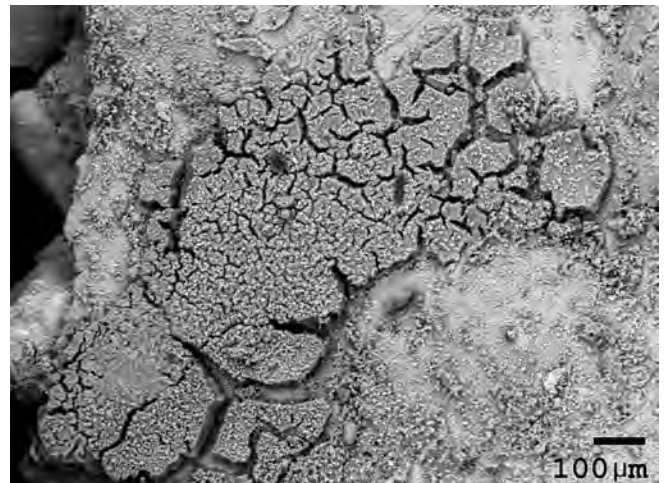
Fig. 5: Scanning electron image of ASR gel in an exposed fracture.
