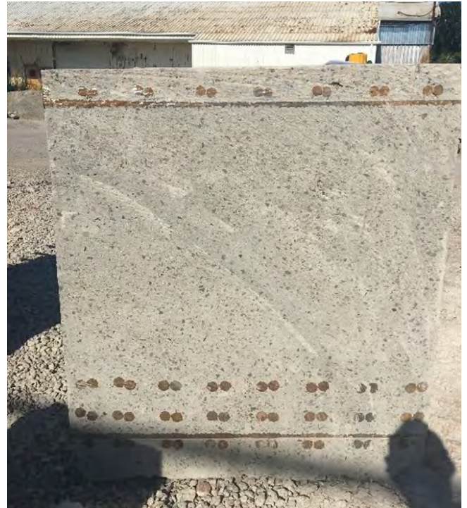
Fig. 21: An example of a wire saw cut section of mockup showing excellent consolidation of shotcrete around the three layers of 35 M rebar at the back of the work and to the outer membrane.
