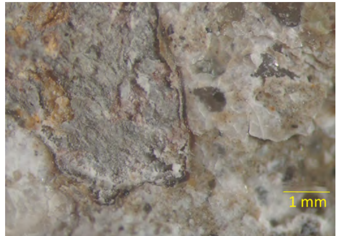
Fig. 1: Photomicrograph of a fresh fracture surface showing a reacted volcanic aggregate with rim development and ASR gel adjacent to the particle.
