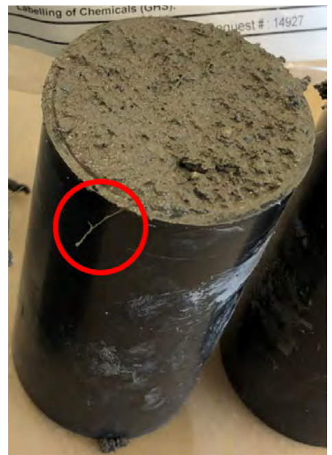
Fig. 1: Photo of unwound kenaf fiber in shotcrete mortar Hardened State Mortar Testing
