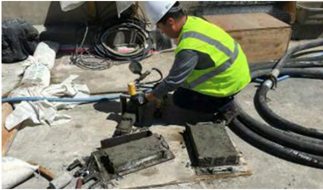
Fig. 8: Early-age compressive strength test
