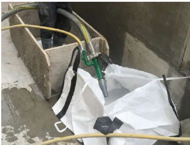
Fig. 3: Green Line G783-200 Fabric Concrete Placement Hose with an inner diameter of 50 mm (2 in.) connected to a nozzle assembly utilizing a unique pipe extension between the rubber nozzle tip and the nozzle air ring. Rubber nozzle tip is wrapped tight with grey duct tape.
