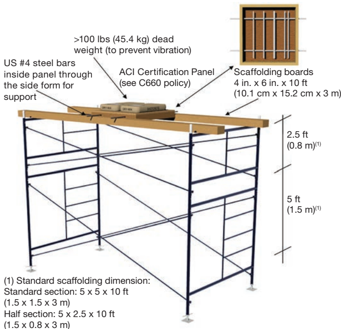
Overhead standard setup—ACI Shotcrete Nozzleman Certification
