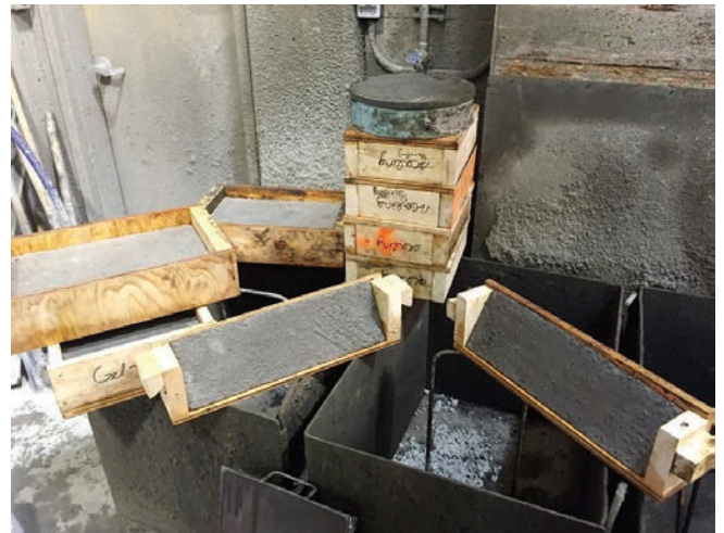
Fig. 4: Inclined precast mold for slant shear bond strength testing (ASTM C882/C882M)
