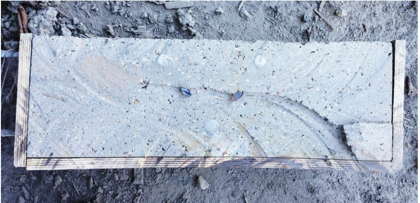
Sawed side of shotcrete test panel shot with multiple layers
