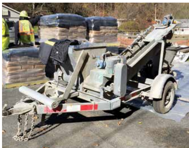
An auger-type pre-dampener used in dry-mix process refractory installations
