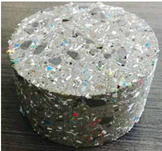
Fig. 7: Shotcrete core containing shredded recycled plastic 14
