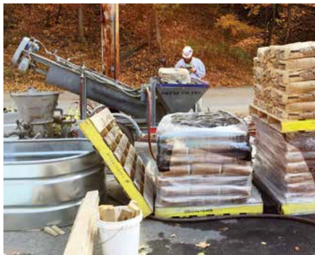
A typical setup used in dry-mix process refractory installations with a rotary gun and an auger-type pre-dampener for gunning dry prepackaged refractory material
