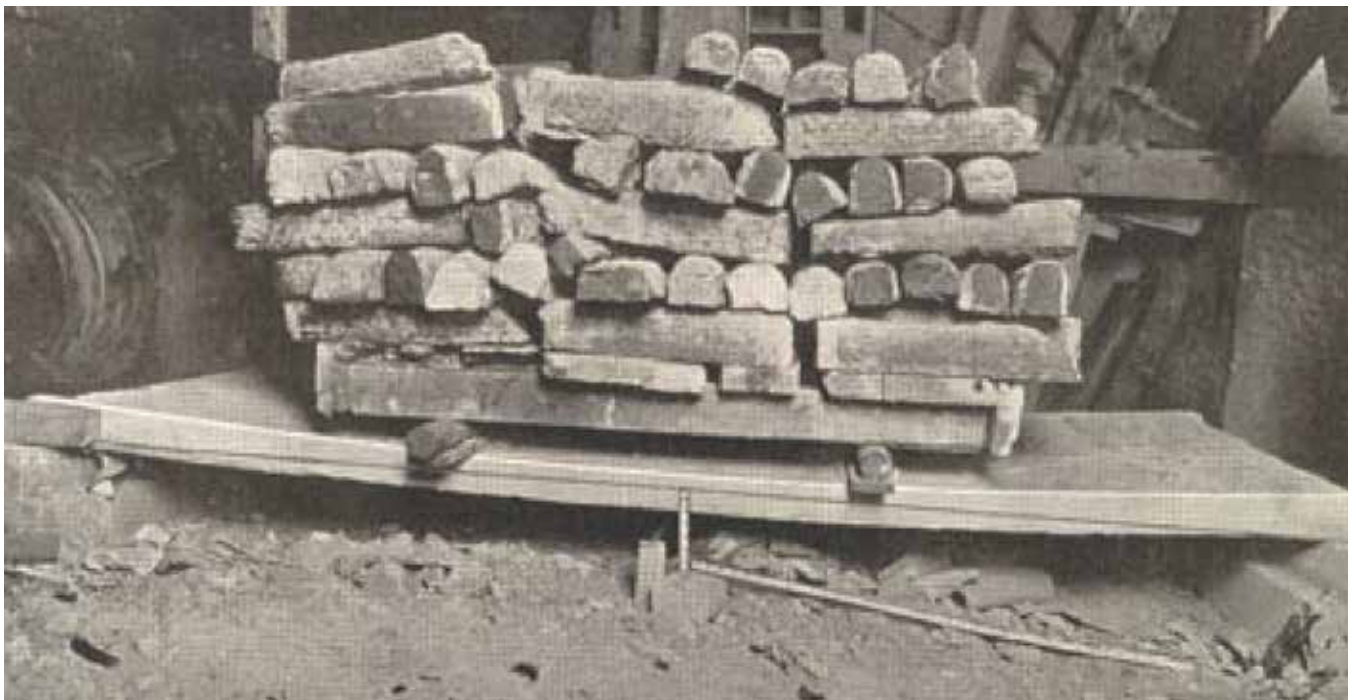
Figure 4. Test of "Gunitite" slabs made under supervision of Prof. M. O. Fuller, Lehigh University. [The tests were started in 1920 and ran through 1934. The 8' 0" (2.4 m) span, 3-1/4" (82.6 mm) thick, deflected 2" (50 mm) by 1922 and stressed the reinforcing to 36,000 lb (160 kN) at completion. No further deflection occurred after the 3rd year.]
