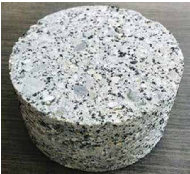
Fig. 8: Shotcrete core containing recycled rubber beads 14
