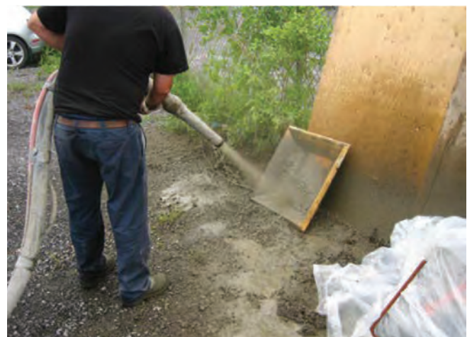
Fig. 6: Preconstruction testing of shotcrete using a test panel
