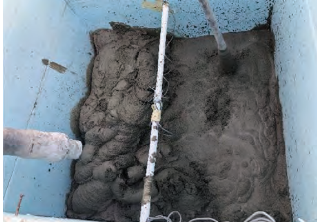
Fig. 3: Casting shotcrete into 1 x 1 x 1 m (3.3 x 3.3 x 3.3 ft) box to calibrate adiabatic temperature rise (ATR).
