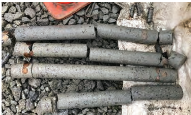
Fig. 5: Cores extracted from mockup wall section.
