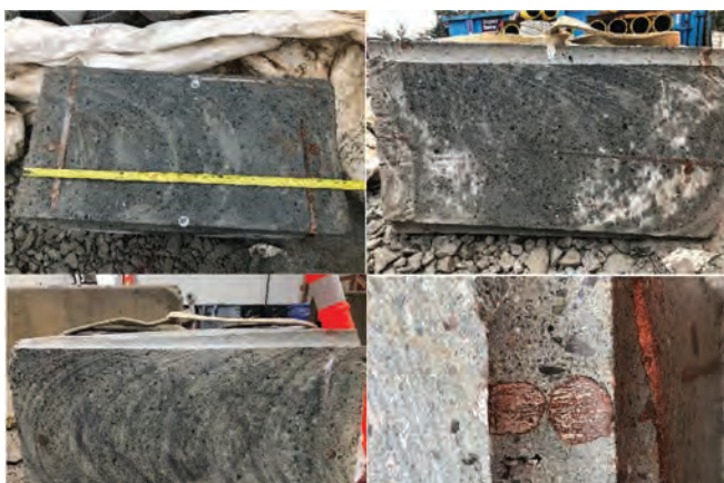
Fig. 6: Cutout block showing thorough shotcrete consolidation around reinforcing bar and cooling pipes.
