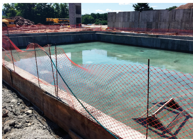
Fig. 3: Watertight tank test
