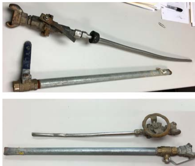
Fig. 1: Non-compliant blow pipe variations.
