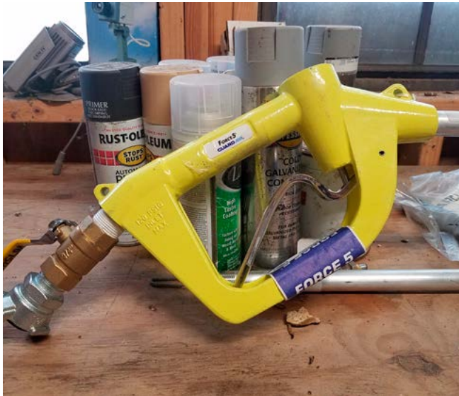
Fig. 3: Dead-man trigger with ball valve installed for volume adjustment.
