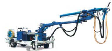
Fig. 5: Typical tunnel electric-hydraulic sprayer.
