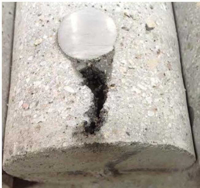
*Fig. 2: This core specimen's major flaw is evidence of inadequate flow during placement.*
