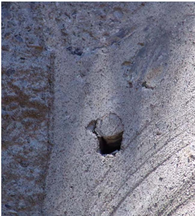
Fig. 4: Void beneath reinforcement in saw cut specimen occurred from downward movement.
