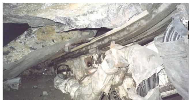
Fig. 1. Rock fall on jumbo equipment
