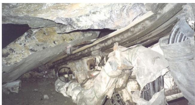
Fig. 1. Rock fall on jumbo equipment
