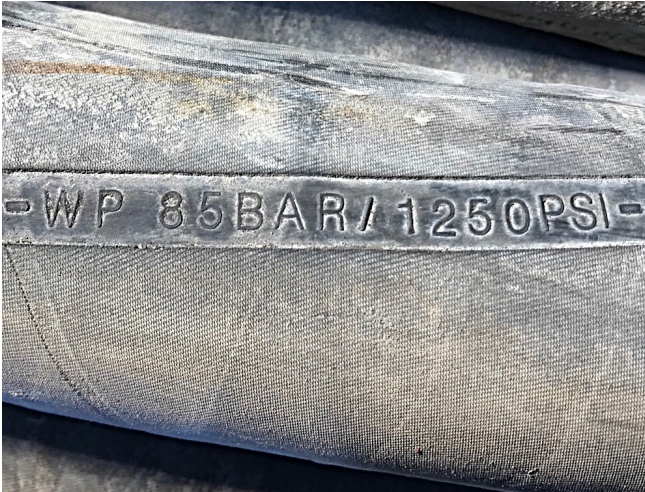
Fig. 3. Working pressure ratings clearly displayed on common placement components.
