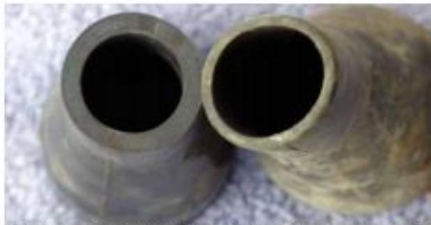
Fig. 6: After placing only 80 lb/ycd (60 kg/m<sup>2</sup>) the worn tip on the right has become oversized and must be discarded
