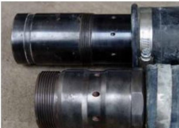
Fig 3: Nozzle body above with 1/8 in. (3.2 mm) drilled ports. Nozzle body below uses 3/16 in. (5mm) ports and adds chamfer to increase air flow
