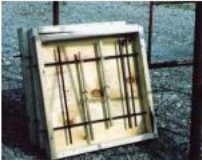
A shotcrete panel form with the simulated reinforcing bars
