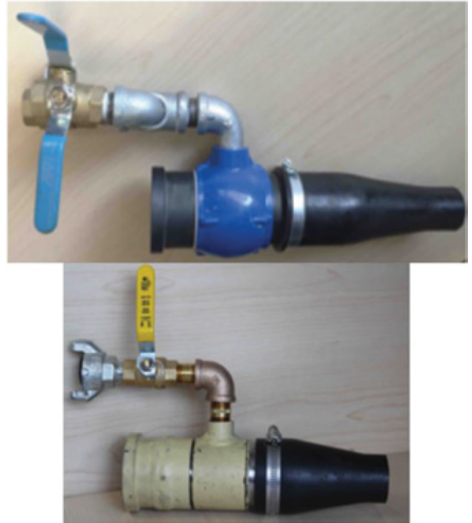
Fig. 3: Tested nozzles during experiments - ACME (top) and 1978 (bottom) (Bérubé, 2017)
