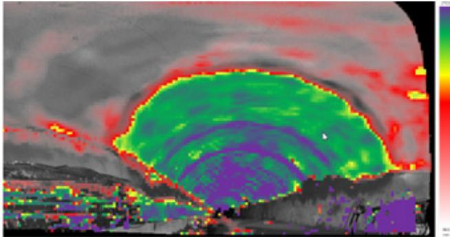
Fig. 14: GML guided spray with zero non-compliant thin spots
