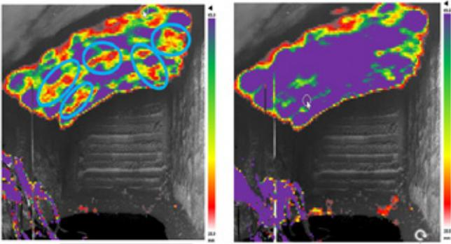
Fig. 8: Detection of overspray and under spray of shotcrete
