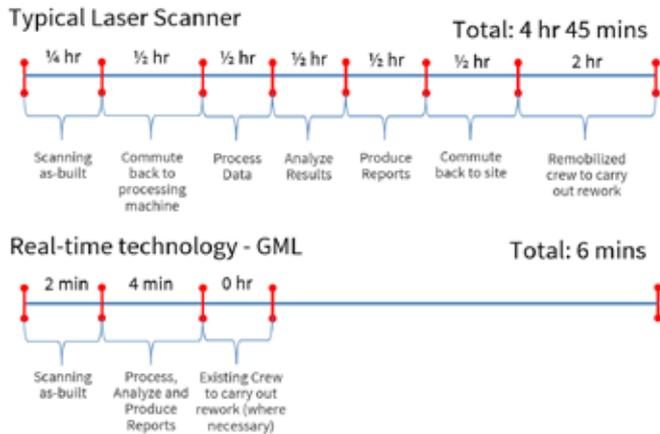
Fig. 3: LiDAR vs In-situ LiDAR Workflow Comparison
