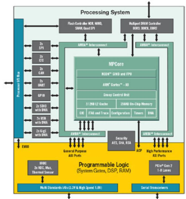
Fig. 2: Xilinx FPGA Architecture
