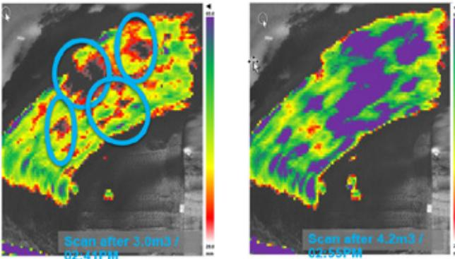
Fig. 9: Nozzlemen guided to fix up thin spots in shotcrete application
