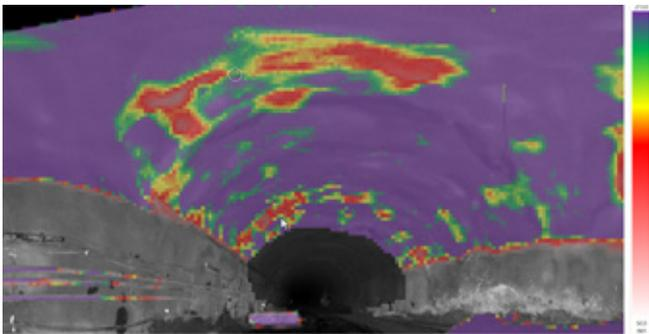
Fig. 12: GML scan showing under spray sections in Red
