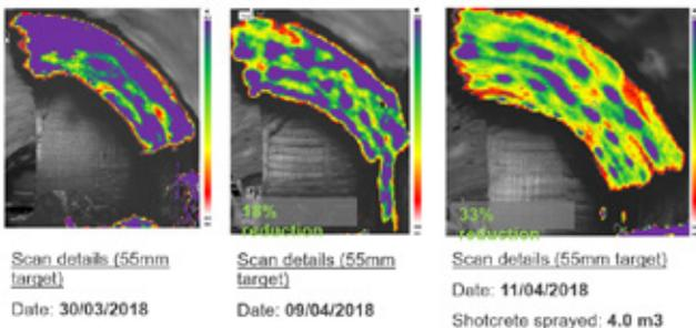
Fig. 10: Reduction of shotcrete usage
