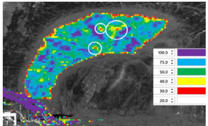
Fig. 13: GML Scan Color threshold for spray thickness
