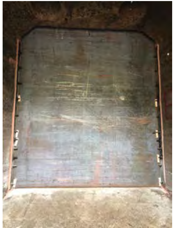
Fig. 1: Temporary safety bulkhead
