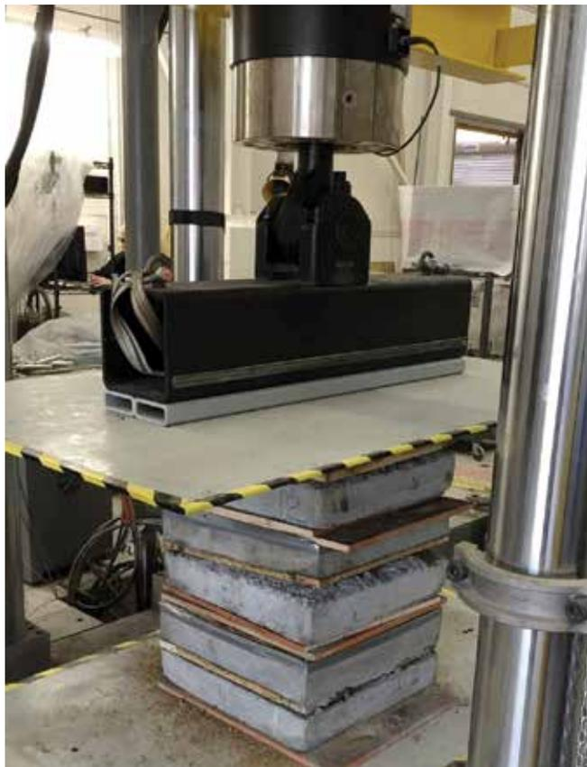
Fig. 4: Composite panels under loading frame
