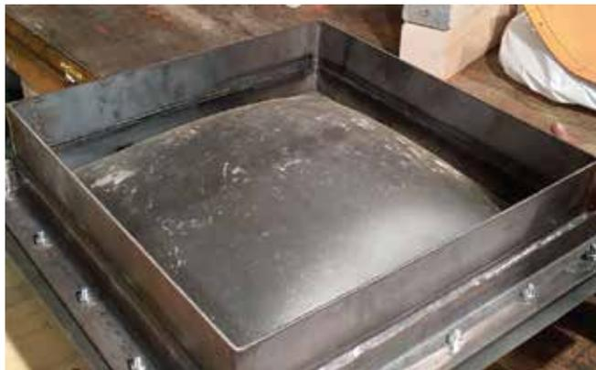
Fig. 9: Inflated membrane at 50 psi of air pressure
