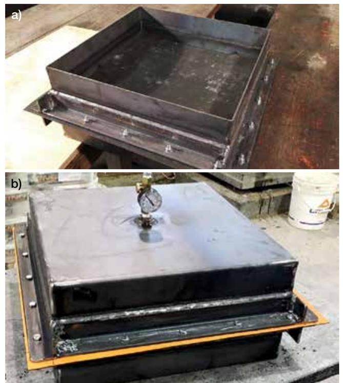
Fig. 5: (a) Testing frame from membrane side; and (b) from air input side
