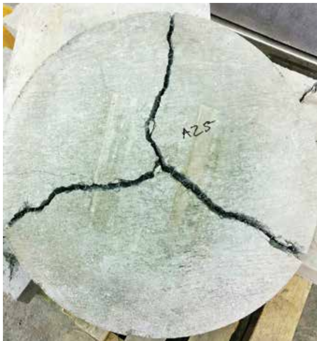
Fig. 2: Typical ASTM C1550 specimen (RDP) after testing
