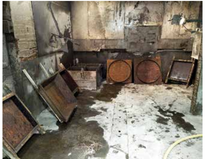
Fig. 3: Large molds to be sprayed with FRS for testing in a research project at Université Laval's Shotcrete Lab
