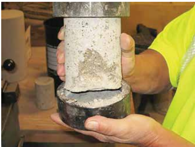
Fig. 3: Type of break indicative of a point load as a result of a core that has not been cut to 90 degrees
