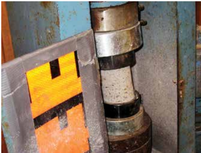
Fig. 2: Specimen that has not been cut to 90 degrees in a break machine
