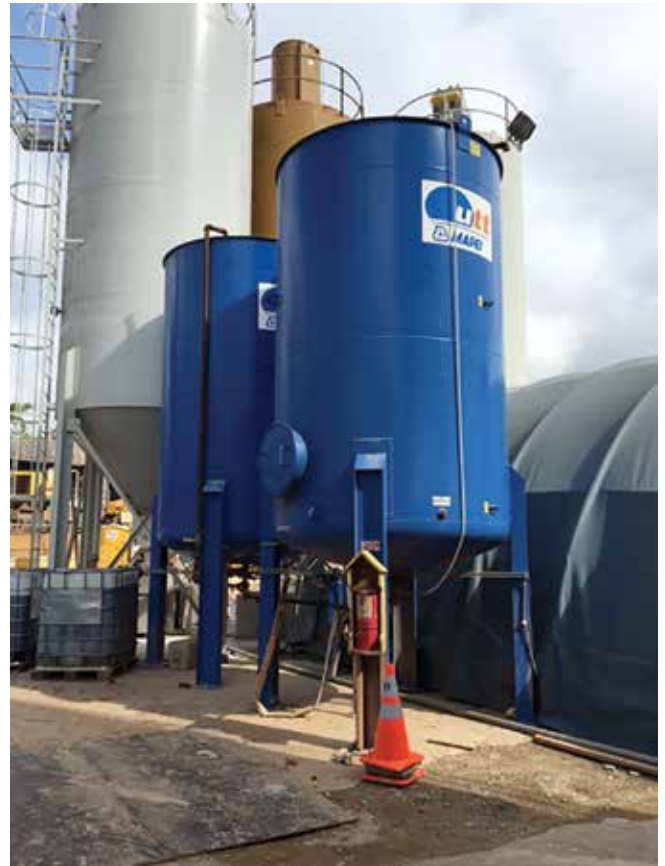
Fig. 3: Mapequick CBS 2 Holding Tanks
