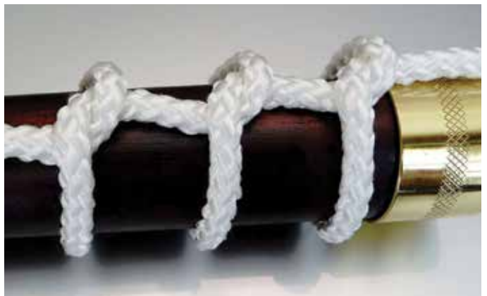
Fig. 2: (a) Overhand knot; and (b) adding two overhand knots, also known as Marline Hitching, above the slipknot gives you a combination that is OSHA-compliant
