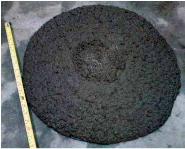
Fig. 10—Typical consistency of 0.45 w/b ratio mixture showing VSI of 0.
