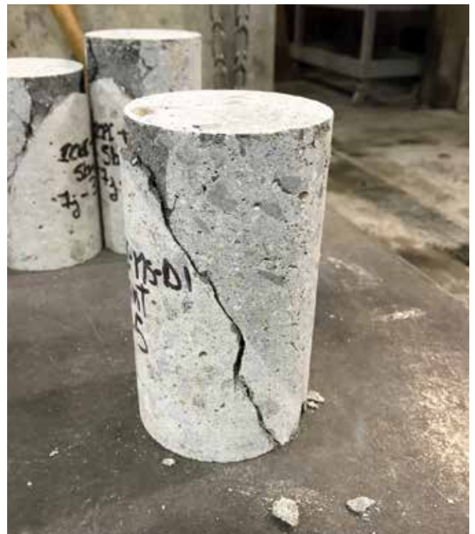
Fig. 5: Composite core for slant shear bond strength testing (ASTM C882/C882M)
