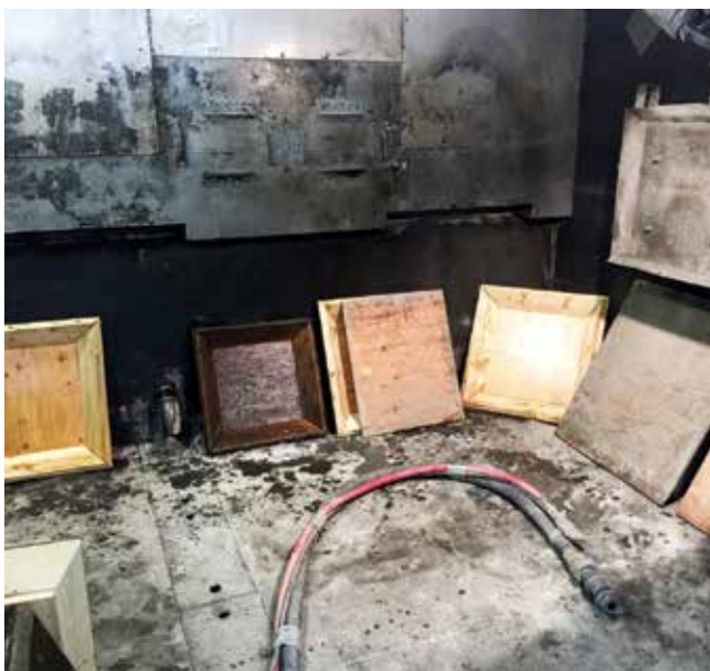
Fig. 2: Conventional square shotcrete test panels used for obtaining cores
