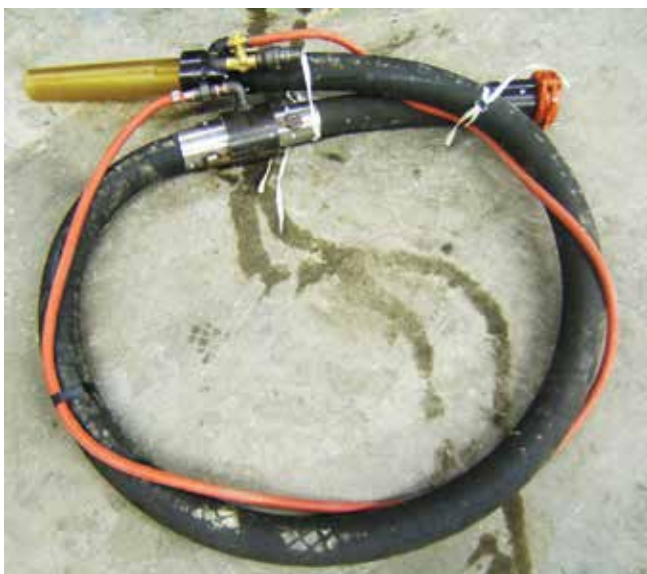
Fig. 1: A 2 in. (50 mm), 8 to 10 ft (2.4 to 3.0 m) hydro-mix nozzle and hose setup that gives good mixing action before the concrete material reaches the nozzle tip. Also, note the easy access to the water body to clean out the water ring daily
