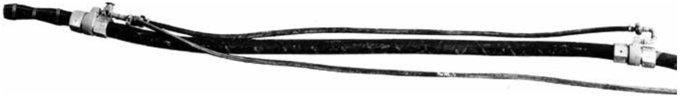
Fig. 2: A prewetting setup with two water valves and nozzle bodies with water rings
