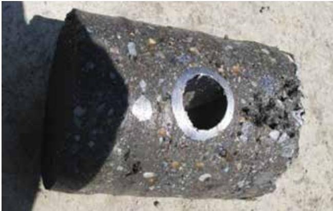
Fig. 14: Side view of Core No. 4. Note porous shadow behind cooling pipe. Assigned ACI Core Grade No. 3
