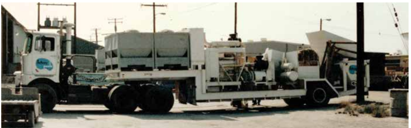
One of Anthony Pools' shotcrete rigs with proportional mixer, Sidewinder pump, diesel generator to run the mixer, hydraulic power to run the concrete pump, and a 350 CFM compressor
