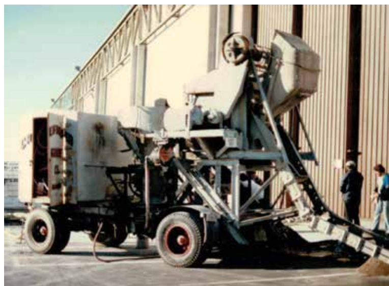
Gunite machine used in Beverly Hills by Anthony Pools when we were invited to inspect their operation. These machines were “dust producers.” In today’s market, the EPA would fine any company using such machines
